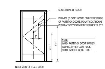
COAT HOOK MOUNTING DETAIL A4.03 | SCALE: 1/4" = 1'-0"
