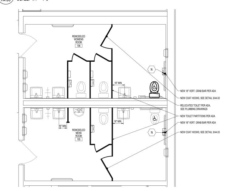
2 REMUDELLE SCALE: 1/4" = 1'-0" REMODELED CUSTOMER RESTROOM DETAIL PLAN
